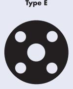
Type E is a full-faced gasket with the same outside diameter as the flange and precision cut bolt holes.
