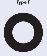
Type F gaskets are made to fit the raised face portion of the flange only. As there are no bolt holes in the F gasket, the outside diameter of the gasket falls within the inside diameter of the bolt hole circle. Available in the same materials as the type E gasket.
